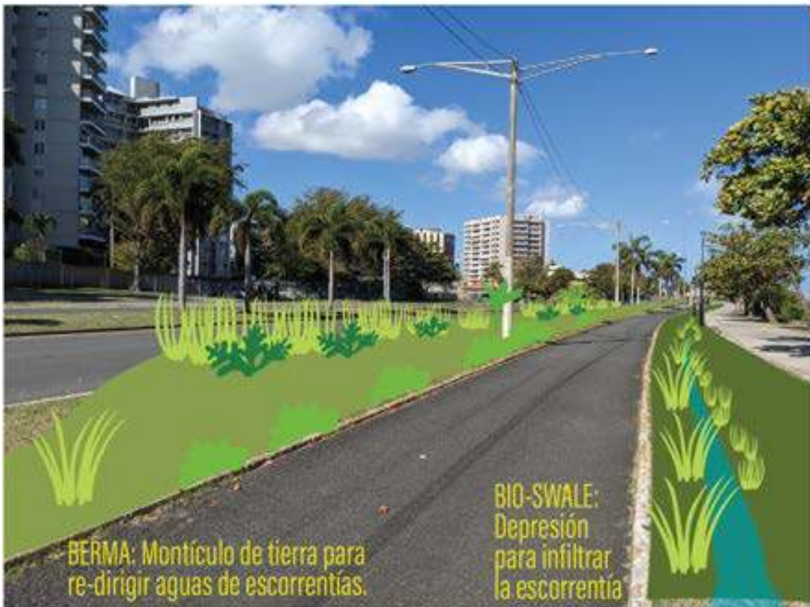
Figure 55. Conceptual green infrastructure design, berms and bio-swales, at Baldorioty Avenue at entrance to Jaime Benitez Park.
