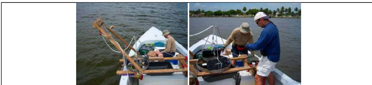
Figure 6. Sediment Sampling Rig Including Petite Ponar Dredge Mounted on Stabilizing Frame. The dredge was lowered by the side of the boat using a portable pulley and frame system constructed for this study. The system allows for the retrieval of sediment and collection of sediments in glass bowls and can be easily installed in different small boats.
